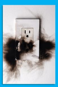
When excessive heat builds up in an outlet, it can melt insulation that covers the wires. Electricity running through exposed wires
